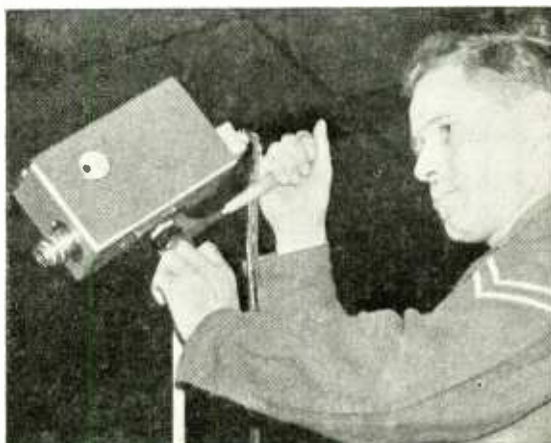
Marconi miniature camera for industrial television.
