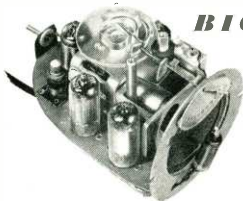
The Faras bicycle receiver and batteries. No space is wasted, as the enlarged interior view on the left shows. The tuning indicator is in front of the loudspeaker.
