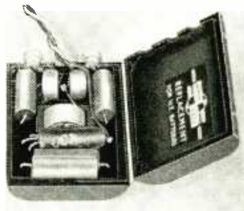
Open view of transistor h.t. generator — the interior is normally filled with potting resin.
