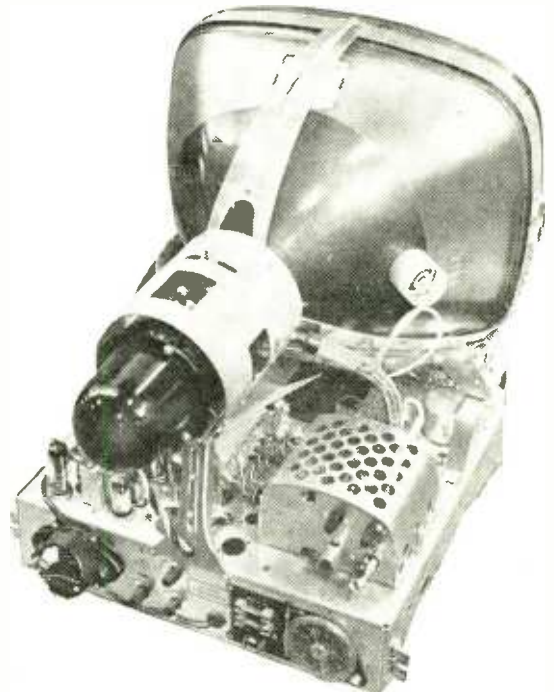
Murphy chassis. Note the thorough screening of the line timebase, the deflector-coils and the inter-connecting leads.
