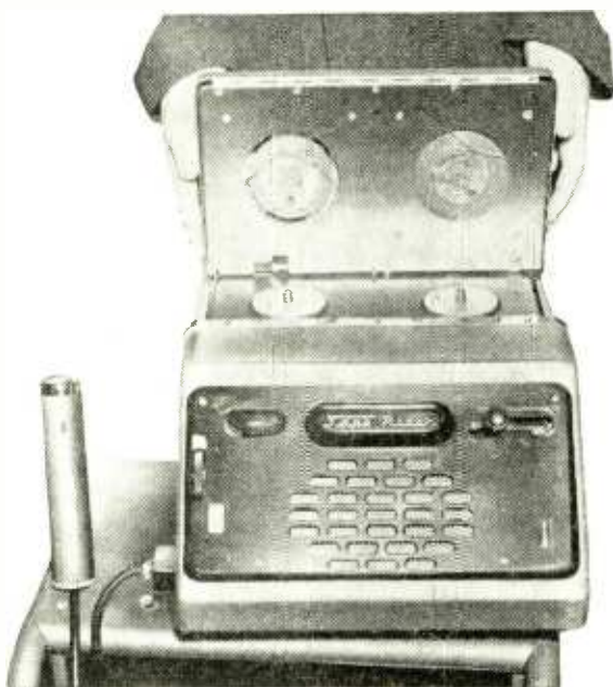
Hartley "Tape Riter" with cassette loading.
