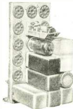
Unit construction in Army pack-set.
